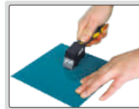
step 1: make grid cutting on surface
