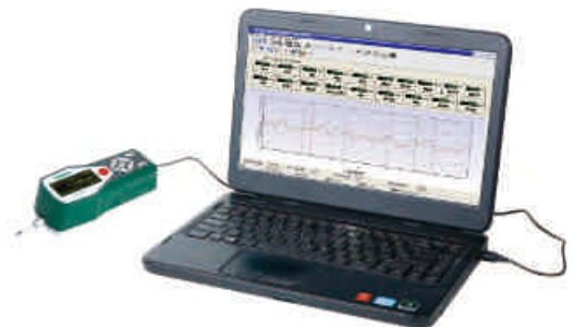
operate roughness tester by computers
