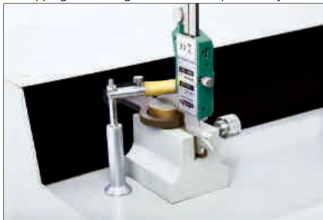
lapping measuring surfaces of caliper lower jaws
