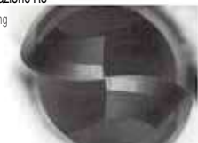
Usura utensile 0.008mm Tool wear
